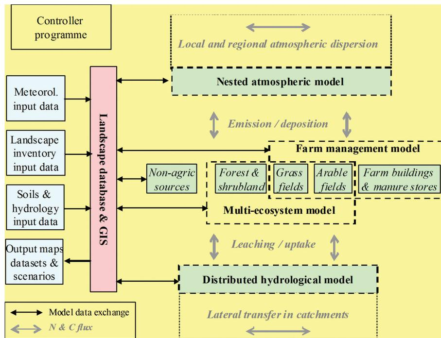
**Figure 11.8** Schematic of the NitroScape modelling framework to provide a fully integrated treatment of N exchange fluxes at the landscape scale. The landscape is envisaged as integrating farms, fields, semi-natural land and non-agricultural sources, with lateral and vertical dispersion fluxes through the atmosphere and hydrosphere (from Sutton *et al.*, 2007).
