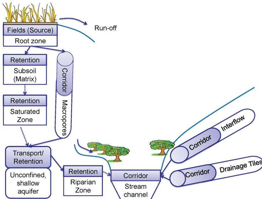
**Figure 11.4** Scheme of corridors and retention compartments. The sequence of compartments depends upon the specific hydrological setting and is spatio-temporally variable (redrawn from Haag and Kaupenjohann, 2001) with permission from Elsevier.
